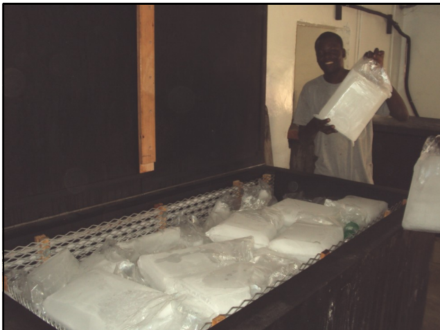
Above: A WISH ice plant employee fills plastic bags with water to be frozen between the refrigeration plates in the ice machine.
