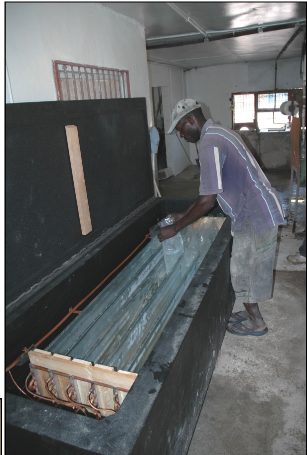
Above: A WISH ice plant employee fills plastic bags with water to be frozen between the refrigeration plates in the ice machine.
